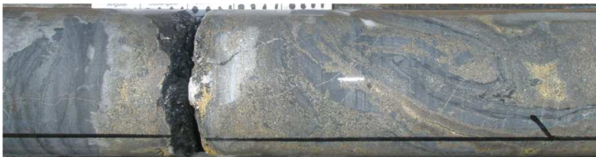
Figure 7 Drill core of zinc mineralisation from JB001
